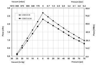
2380 Series Flow at Pressure/Vacuum Curve
